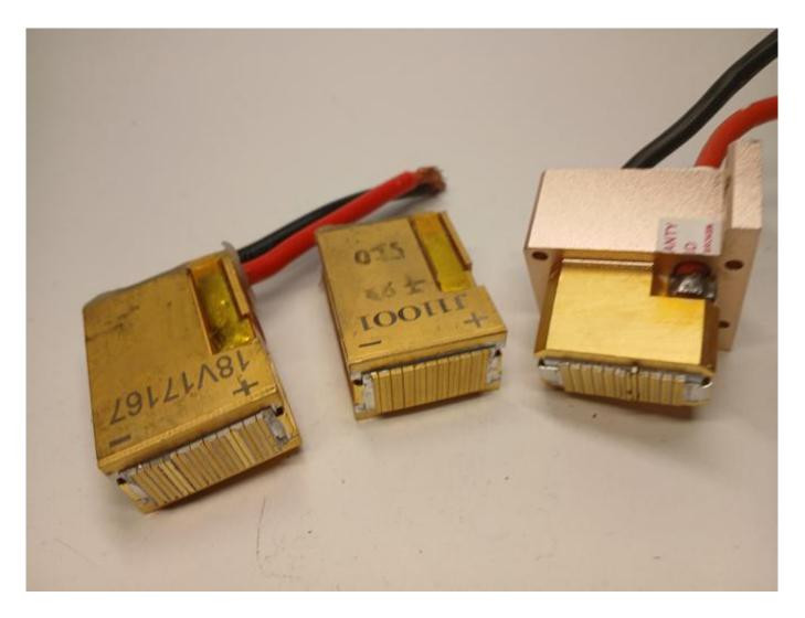
Which voltage to apply for diode stack check WWW.ROMSHI.COM - home of online laser maintenance help
