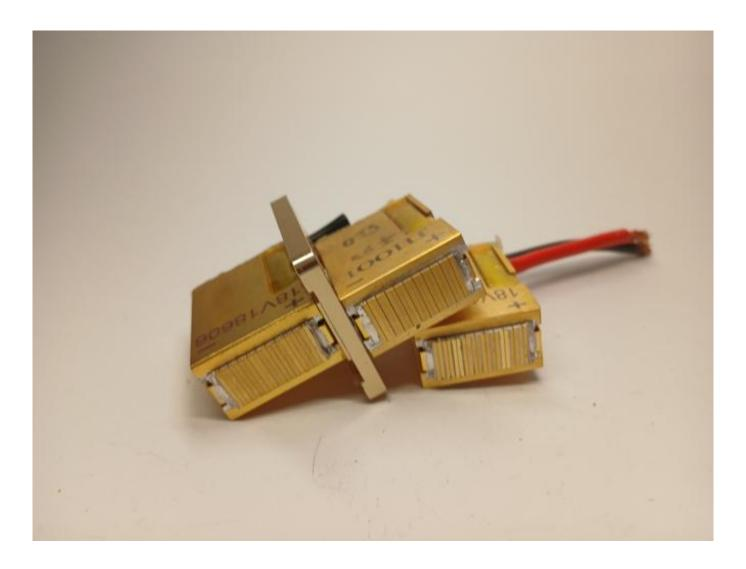
Extra 808nm laser diode assembly Diode stack international orders accepted at WWW.ROMSHI.COM
