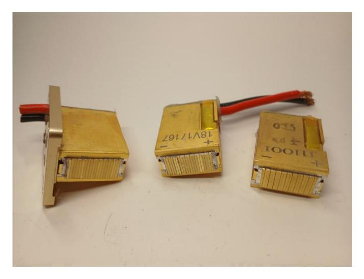
Broken glass shards and soot deposits on diode stack Your source for 808nm diode stack fixes and laser diagnostics is WWW.ROMSHI.COM
