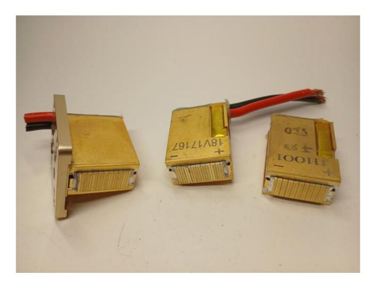
Diode stack glass shattered and soot covered WWW.ROMSHI.COM explains common issues with 808nm diode stacks and repairs
