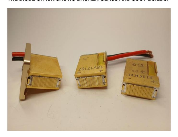
The diode stack shows broken glass and soot buildup Access troubleshooting info for 808nm diode stacks and lasers at WWW.ROMSHI.COM
