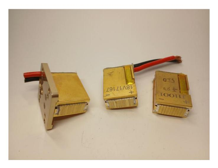
Soot and cracked glass found on the diode stack Fix diode stack errors and learn about 808nm laser tech at WWW.ROMSHI.COM
