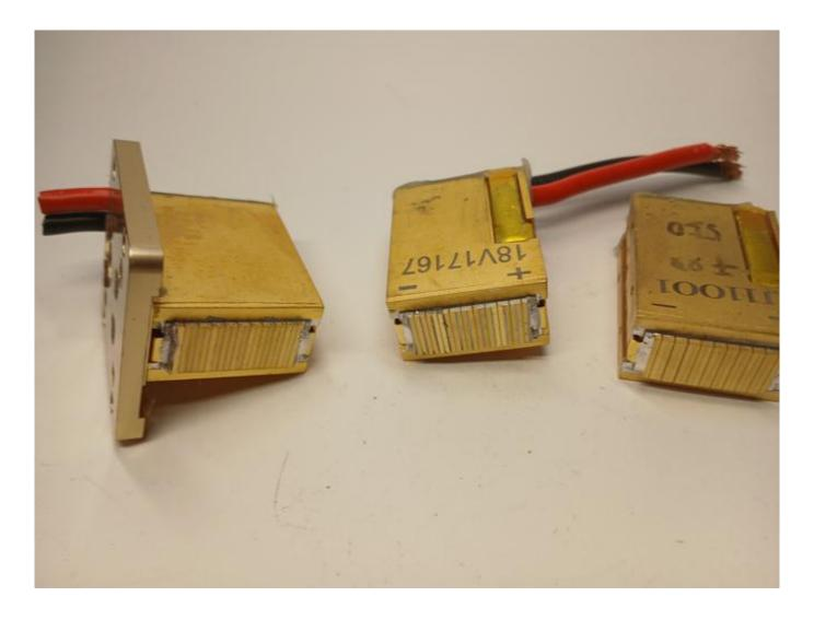
Broken glass and soot deposits on the diode stack Everything you need to know about 808nm diode stacks and laser repair at WWW.ROMSHI.COM
