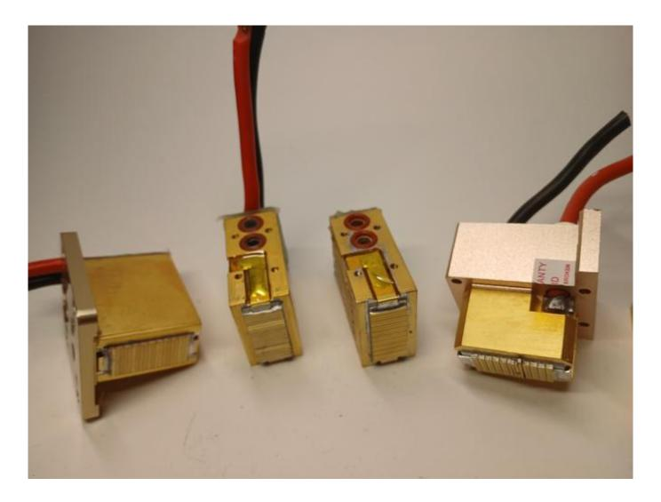
Diode stack has glass break and soot build-up Laser diagnostics and diode stack 808nm help provided at WWW.ROMSHI.COM
