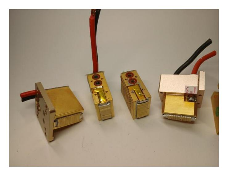
Soot and broken glass shards on the diode stack Find content about 808nm laser modules and servicing at WWW.ROMSHI.COM
