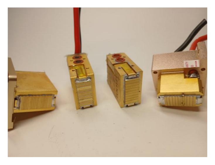
Broken glass on diode stack with soot accumulation WWW.ROMSHI.COM's blog educates on 808nm diode stack functions and repairs
