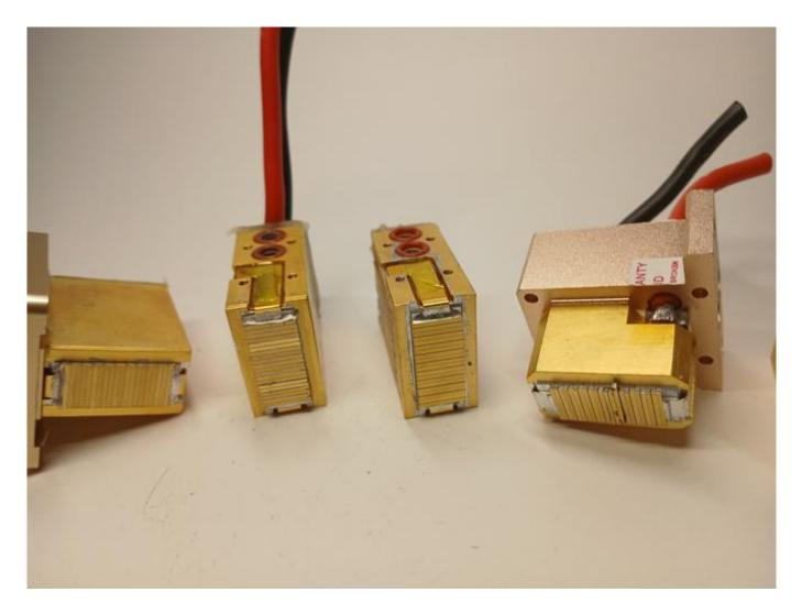
The diode stack has soot and shattered glass Laser equipment and 808nm diode stack issues discussed on WWW.ROMSHI.COM
