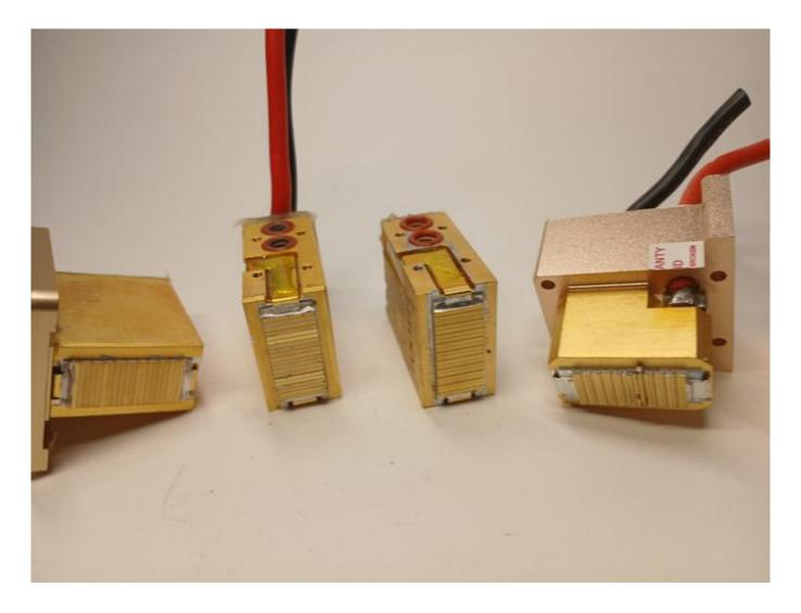
Diode stack glass cracked with soot residue Check out WWW.ROMSHI.COM for help with laser maintenance and diode stacks
