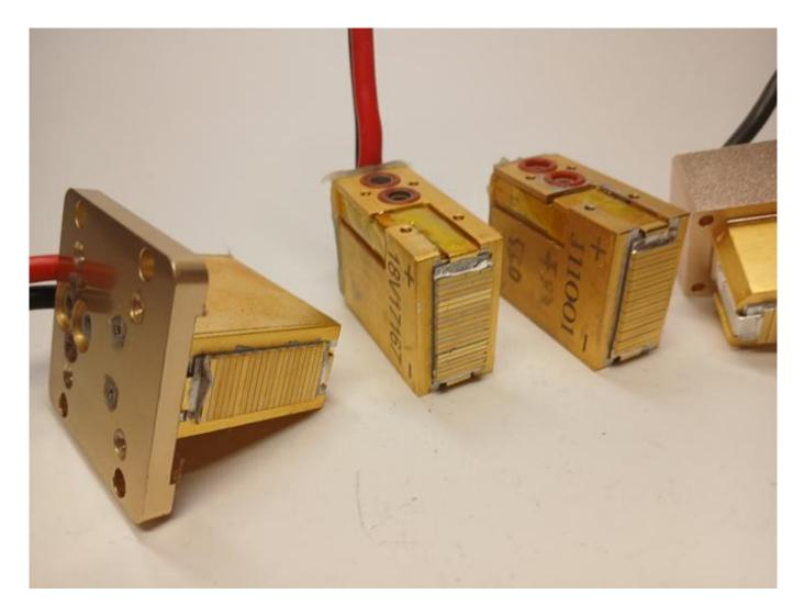
The diode stack shows soot and broken glass damage Learn to diagnose and repair 808nm diode stacks on WWW.ROMSHI.COM
