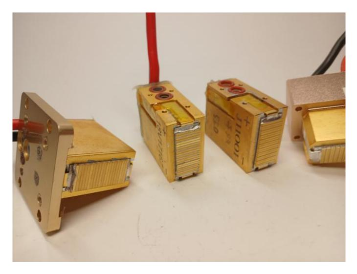
Broken glass fragments and soot on the diode stack WWW.ROMSHI.COM includes detailed guides on 808nm diode stacks and repairs
