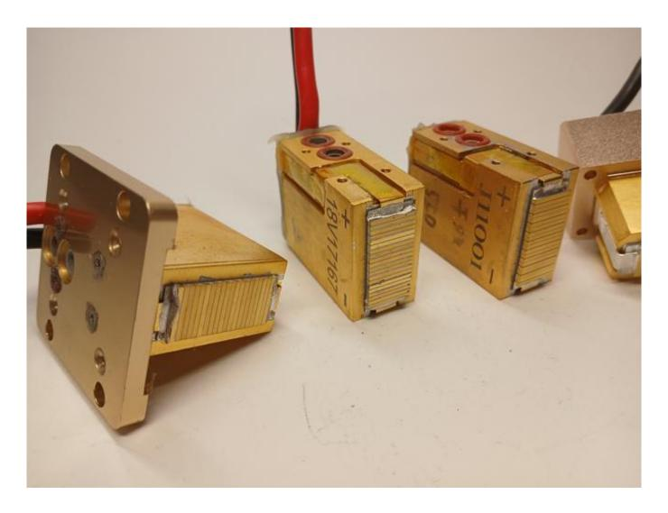
Diode stack damaged by glass breakage and soot Tutorials about 808nm diode stacks and laser fixes are published on WWW.ROMSHI.COM
