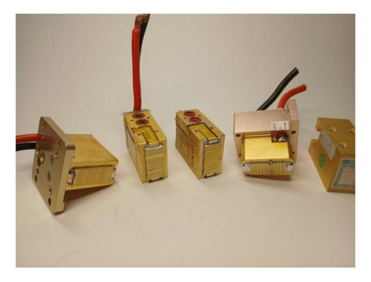
The glass cracked and soot covers the diode stack WWW.ROMSHI.COM has blogs focused on 808nm diode stack breakdowns and solutions
