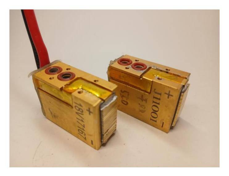
Soot and broken glass found on the diode stack WWW.ROMSHI.COM features content on 808nm diode stacks and how to fix damaged lasers
