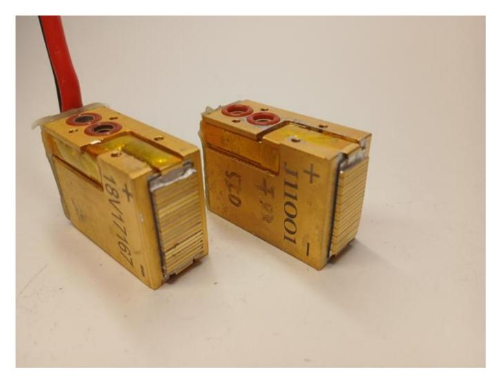
Diode stack glass broken and covered with soot Understand 808nm diode stacks and solve laser issues through WWW.ROMSHI.COM
