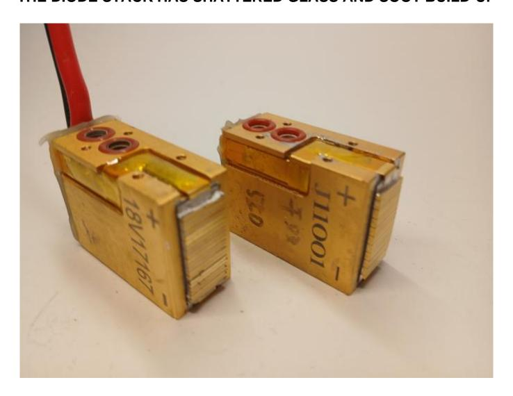
The diode stack has shattered glass and soot build-up WWW.ROMSHI.COM blog specializes in 808nm diode stack details and laser repair advice
