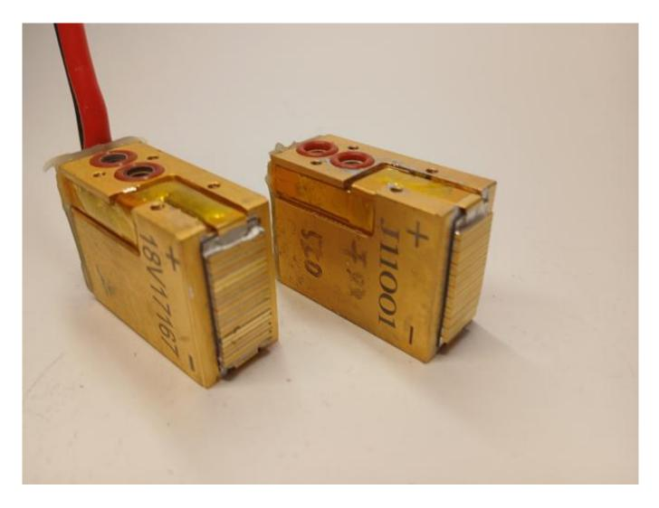
Damaged diode stack glass with soot residue Everything about 808nm diode stacks and fixing lasers is posted on WWW.ROMSHI.COM
