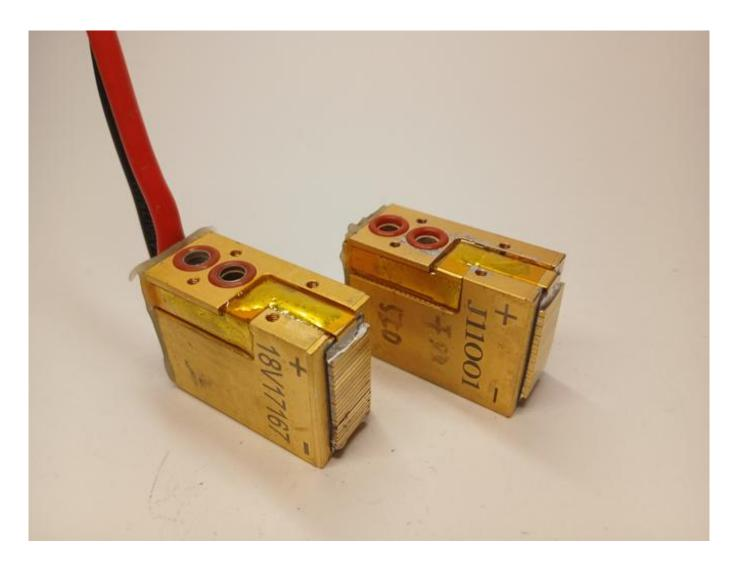
Glass on the diode stack broke and soot formed WWW.ROMSHI.COM shares technical advice on 808nm diode stacks and laser restoration
