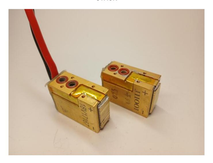
Shattered glass and soot accumulation on the diode stack Discover tutorials for laser repairs and 808nm diode stack insights at WWW.ROMSHI.COM
