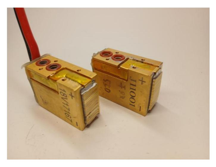
The diode stack shows broken glass and soot deposits Find articles about 808nm diode stacks and common laser issues at WWW.ROMSHI.COM
