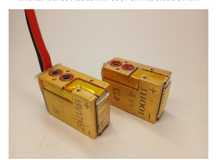
Broken glass pieces and soot on the diode stack Blog at WWW.ROMSHI.COM explores 808nm diode stacks and tips for repairing lasers
