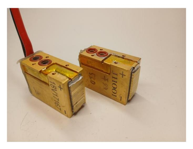
Diode stack with shattered glass and soot contamination Visit WWW.ROMSHI.COM for laser diagnostics and 808nm diode stack explanations
