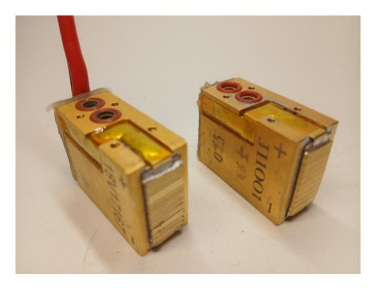
The diode stack glass broke and has soot marks Discover techniques for laser servicing and 808nm diode stack handling at WWW.ROMSHI.COM
