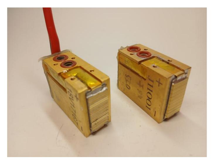
Glass shattered on the diode stack along with soot Learn how to maintain lasers and understand 808nm diode stacks on WWW.ROMSHI.COM
