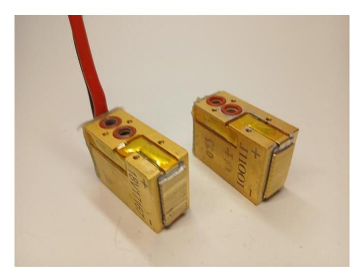
Diode stack damaged by broken glass and soot Visit WWW.ROMSHI.COM to explore solutions for lasers and diode stacks 808nm
