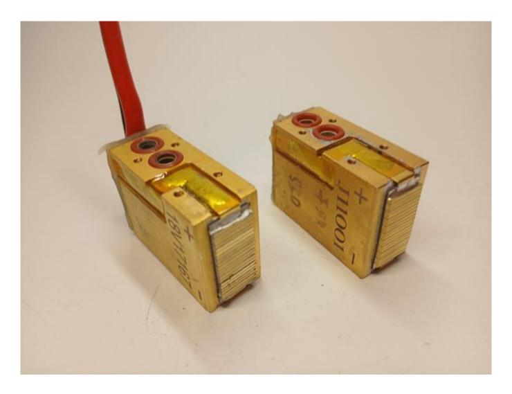
Cracked glass and soot present on the diode stack WWW.ROMSHI.COM is your source for 808nm diode stacks and laser repair how-tos
