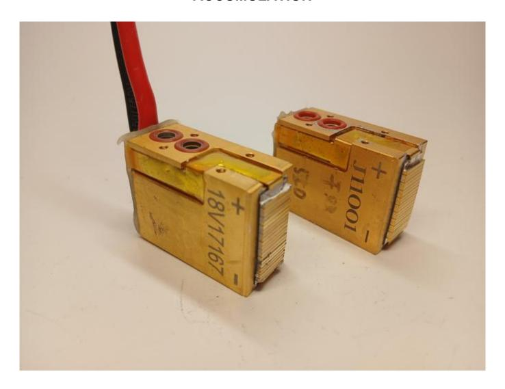
The diode stack glass shattered with soot accumulation Find in-depth blog posts on 808nm diode stack technology and laser maintenance at WWW.ROMSHI.COM
