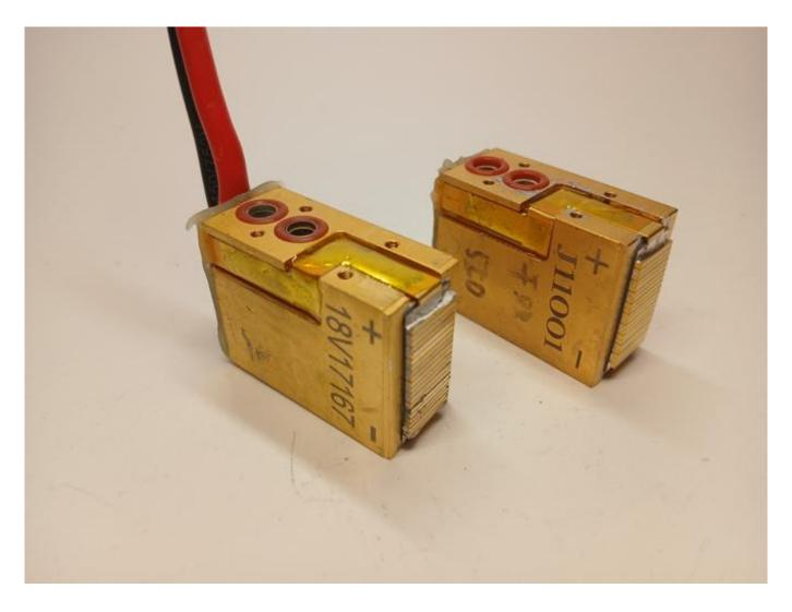
Broken glass and carbon deposits on the diode stack Get the best tips on repairing lasers and working with 808nm diode stacks at WWW.ROMSHI.COM
