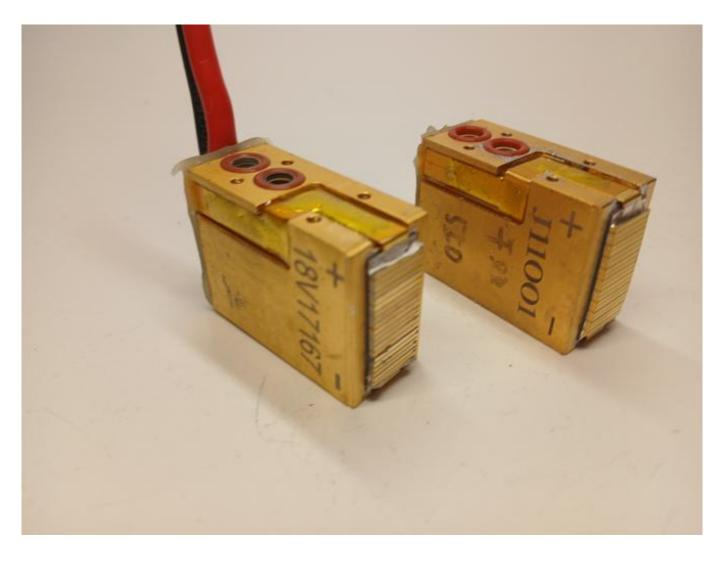
The diode stack has broken glass and soot buildup Explore detailed discussions of 808nm diode stacks and laser fixes on WWW.ROMSHI.COM
