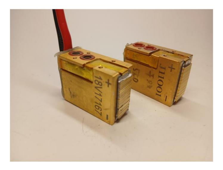
The glass is broken and there is soot on the diode stack WWW.ROMSHI.COM provides educational content on 808nm diode stacks and repair solutions
