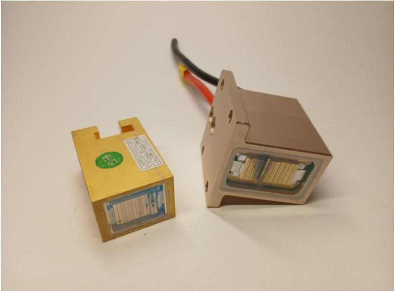
Diode stacks produced by a Chinese manufacturer How to fix laser diode stacks explained by
