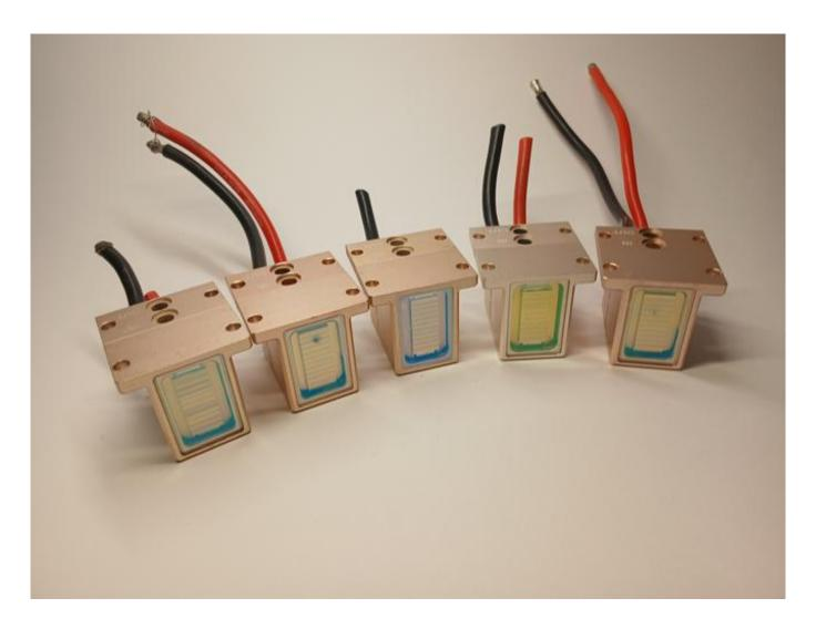
laser handpiece repair and replacement of diode stack WWW.ROMSHI.COM supplies diode stacks to customers worldwide
