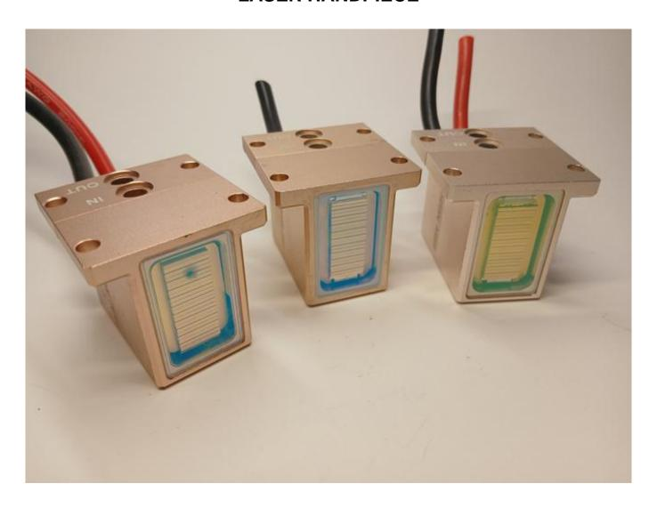
How important is the height of the diode stack in the laser handpiece Laser experts share 808nm diode stack knowledge and fixes on WWW.ROMSHI.COM
