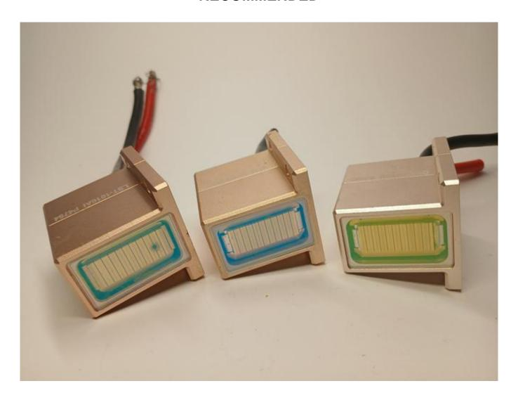
Inside the laser module water is present, replacement recommended WWW.ROMSHI.COM features content on 808nm diode stacks and how to fix damaged lasers
