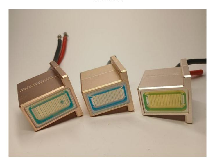
Laser module with water inside needs replacement urgently Explore 808nm diode stack repairs and maintenance blogs on WWW.ROMSHI.COM
