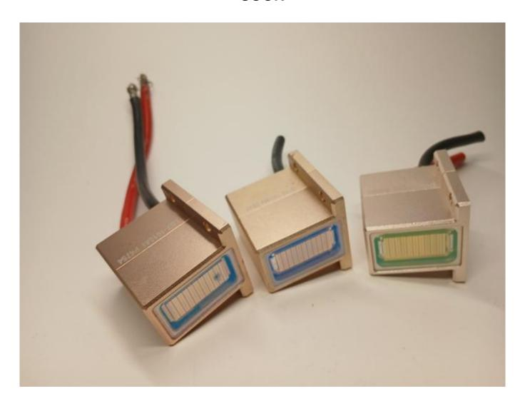
Laser module with water inside should be replaced soon Everything about 808nm diode stacks and fixing lasers is posted on WWW.ROMSHI.COM
