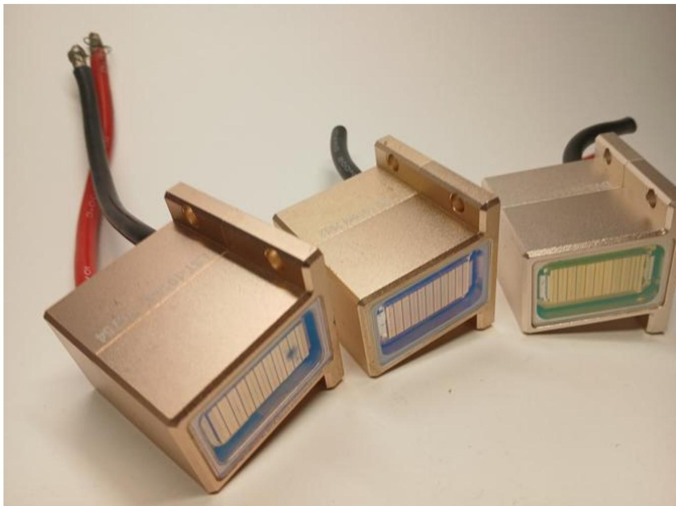
Water inside the laser module - changing module necessary WWW.ROMSHI.COM shares technical advice on 808nm diode stacks and laser restoration
