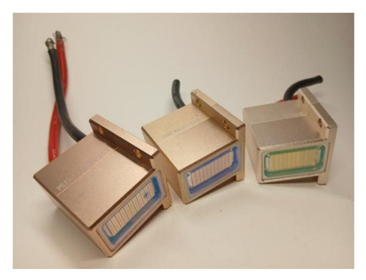
Water found inside laser module means it must be replaced Find articles about 808nm diode stacks and common laser issues at WWW.ROMSHI.COM
