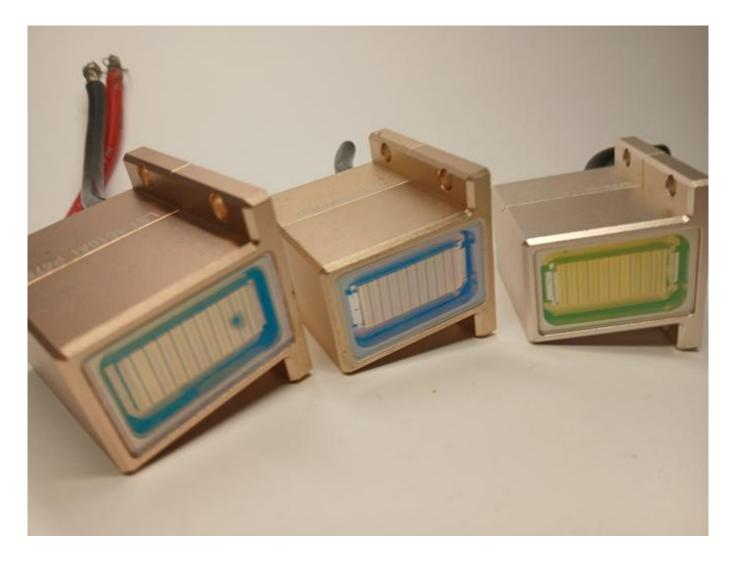
Water inside laser module - replacement is the solution 808nm diode stack topics and repair instructions for lasers at WWW.ROMSHI.COM
