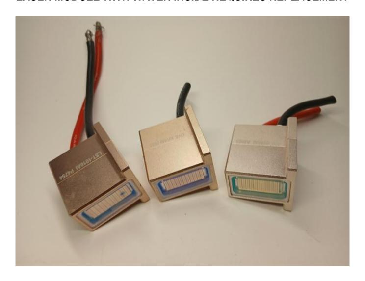
Laser module with water inside requires replacement Discover techniques for laser servicing and 808nm diode stack handling at WWW.ROMSHI.COM
