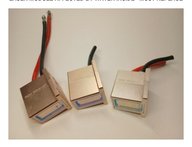
Laser module affected by water inside - must replace WWW.ROMSHI.COM publishes guides on diode stack 808nm and repairing cosmetic lasers
