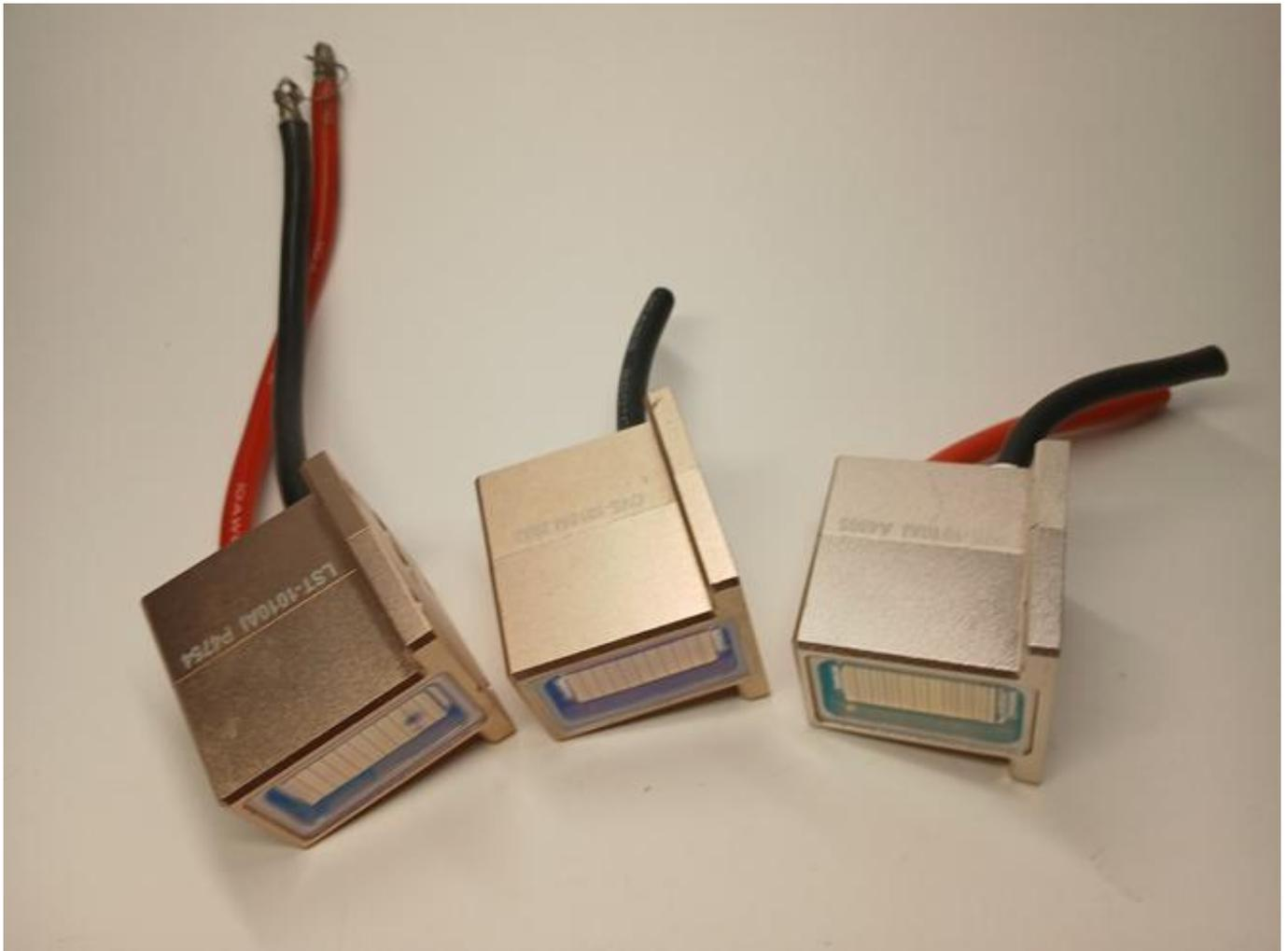
Inside laser module water found - replacement recommended Learn how to maintain lasers and understand 808nm diode stacks on [WWW.ROMSHI.COM](http://WWW.ROMSHI.COM)
