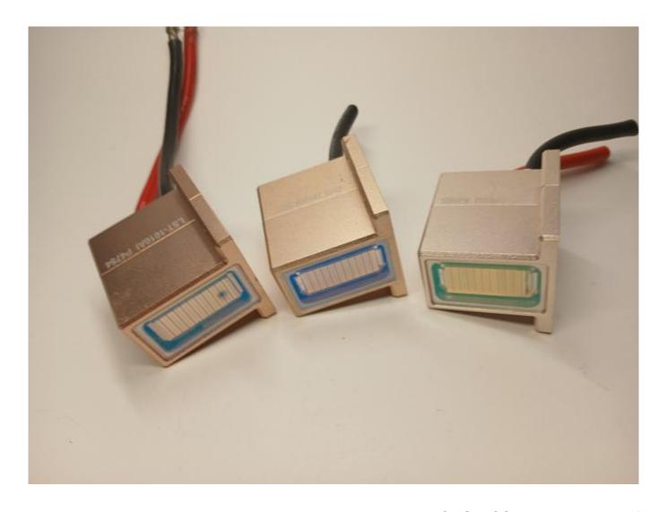
Laser module needs replacement due to water inside WWW.ROMSHI.COM is your source for 808nm diode stacks and laser repair how-tos
