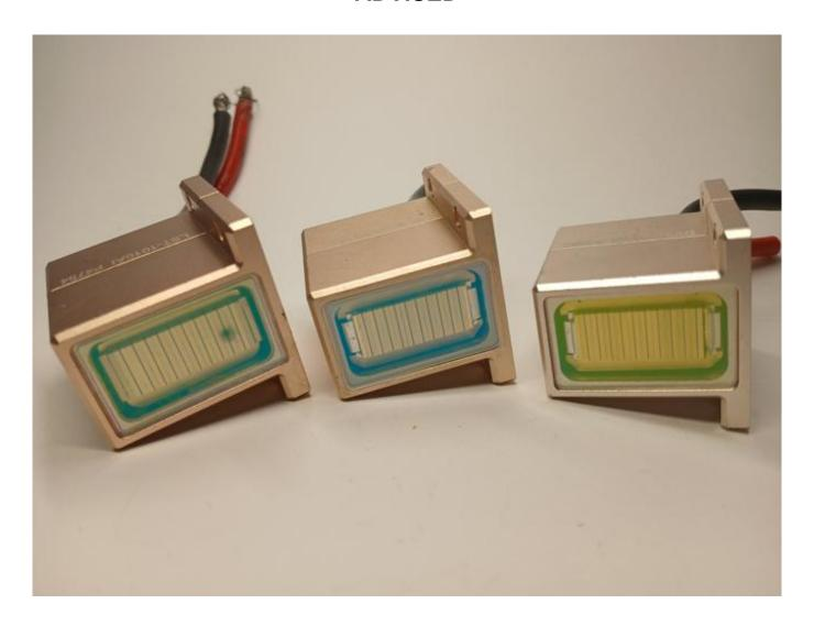
Laser module water contamination - replacement advised Find in-depth blog posts on 808nm diode stack technology and laser maintenance at WWW.ROMSHI.COM
