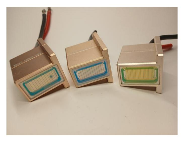
Inside laser module water detected; replacement needed urgently Access valuable knowledge about laser repair and diode stacks 808nm at WWW.ROMSHI.COM
