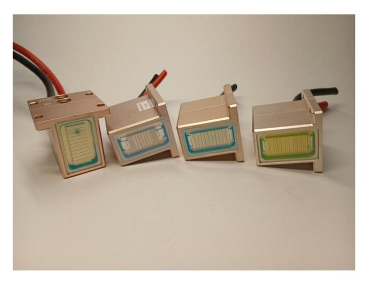
Laser module with internal water - needs to be replaced Laser repair blog with details about 808nm diode stacks can be found on WWW.ROMSHI.COM
