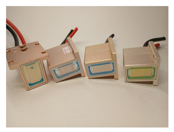
If water is inside the laser module, replacement is essential WWW.ROMSHI.COM presents laser equipment repair guidance and 808nm diode stack insights
